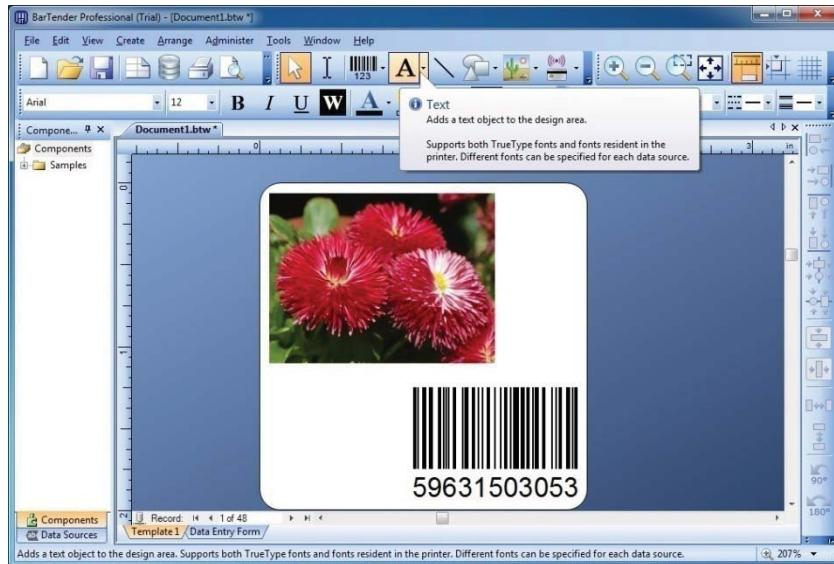
Move the image and the Bar Code as preferred. To add text, click the **Text** button. **Note: When resizing Bar Codes, always use a Bar Code Scanner to verify that the Bar Code remains readable with the correct information.**
