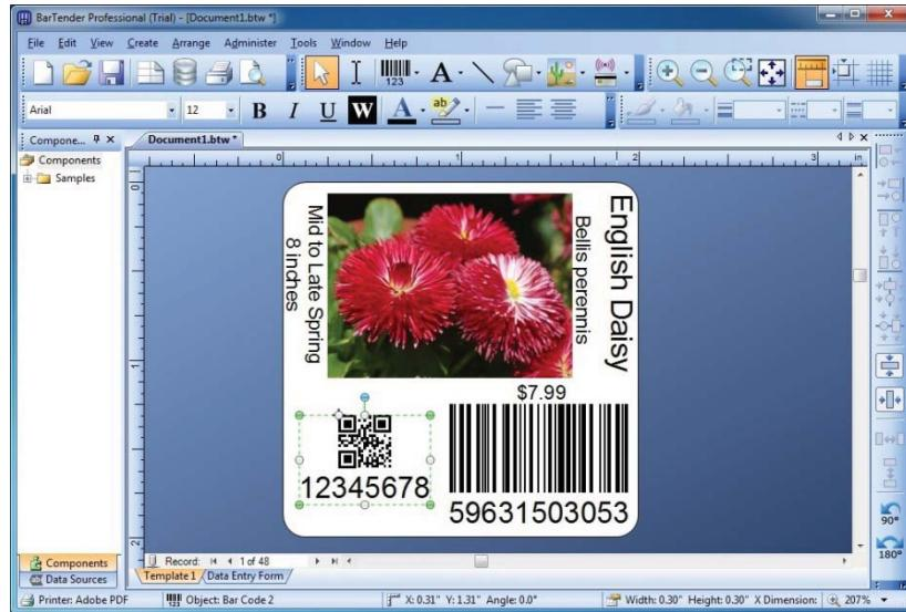
Click to insert Bar Code into the page. Make the necessary Field Name selection and formatting adjustments to the Bar Code.
