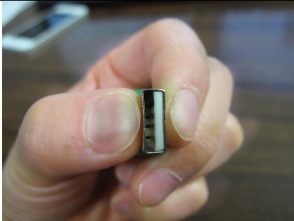
Disconnect your green dongle from your computer, use your finger to squeeze the metallic part a little bit to make the connection better. Insert the green dongle to the computer.
