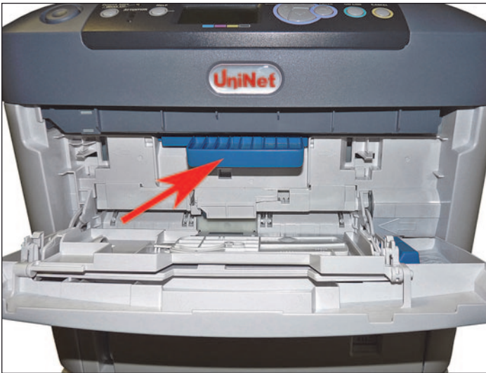
8. Pull down on the blue handle to open the inner door.
