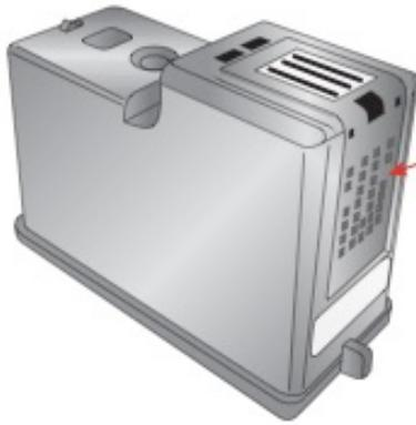
**DRY EXCESS WATER FROM CARTRIDGE. ENSURE CARTRIDGE CONTACTS ARE COMPLETELY DRY. PRINTER DAMAGE MAY RESULT IF CARTRIDGE CONTACTS ARE NOT COMPLETELY DRY.**
