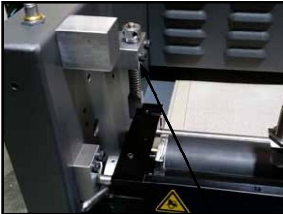
Figure - Coating Unit Spring Rod Mounting Bolts
