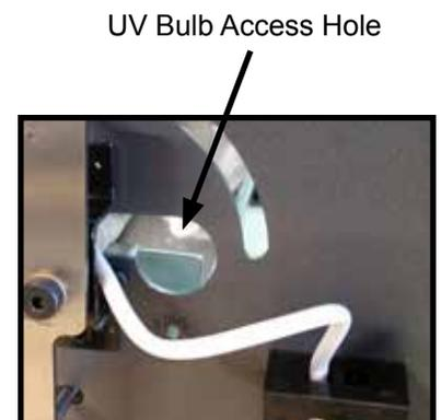
Figure - Bulb Disconnect (UV bulb access cover removed)
