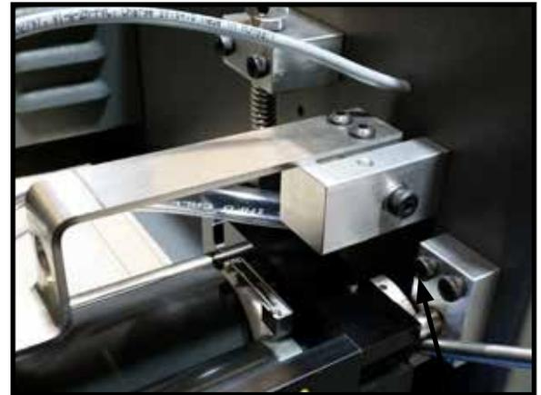
Figure - Coating Unit Mounting Pivot Bolts
