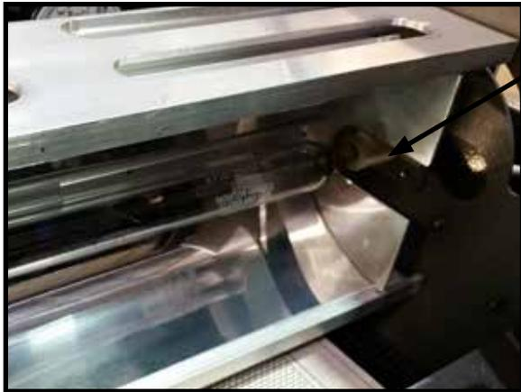
Figure - Rotated UV Reflector with Heat Sink Removed
