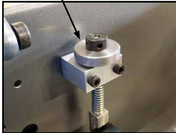
Figure - Form to Impression Roller Pressure
