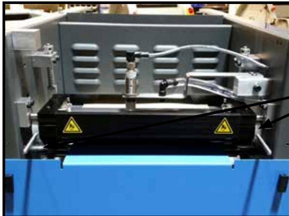
Coating Unit Metering Gauge Adjustment
