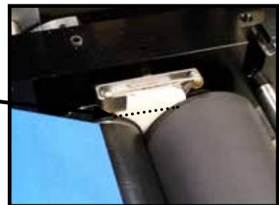
Figure - Coating Fill Line
