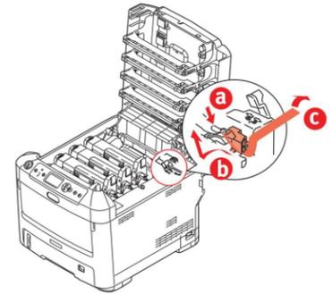
3. Uninstall the cartridges to remove the protective orange film from each. Lock the blue lever forward. Reinstall the cartridges.
