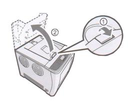
2. Remove the white toner cartridge. Remove protective foam from inside the machine and protective film from the white cartridge and reinstall.
