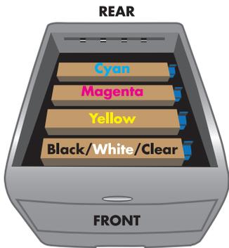
For **Underprinting** white. Typically used for right side reading applications like printing color on clear or dark medias
